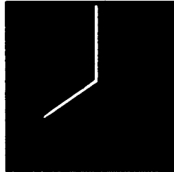
Diode paralleled by 680Ω
